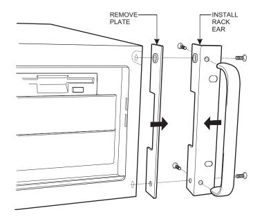
Figure 1. Rack Ear Installation
